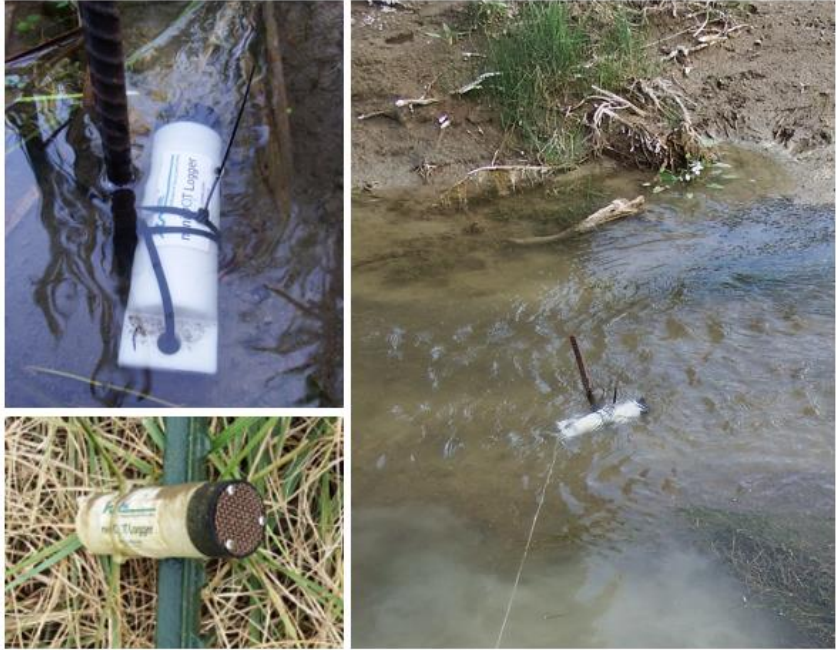
Figure A-3. Dissolved Oxygen Sonde Deployment.
